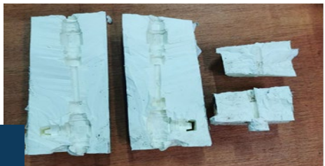
Solidified TAS removed from test fixture after 24 hrs curing
