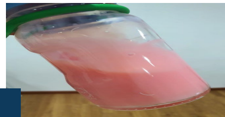
PAS in liquid form — multiple viscosity grades (25 / 200 / 500 cp)
